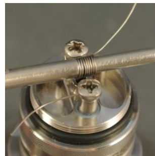
Pic. 4: Adjust the coil with the winding aid.
