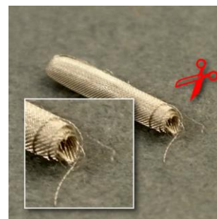
Pic. 4: If the mesh becomes frayed at the edges, it is recommended to remove these thin threads with scissors.
