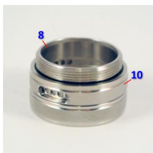
Pic. 13: The o-ring [9] holds the AFC-ring [10] in place.
