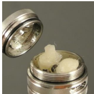
Pic. 6: If you open the chamber again to access the coil, it may happen that the cotton wicks remain hanging on the coil.
