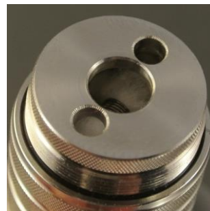
Pic. 16: When you look through the wick holes, you should see the batting.
