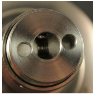
Pic. 2: You can see the cotton through the wick holes..
