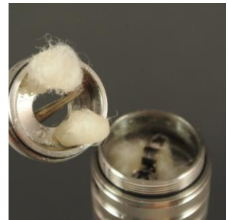
Pic. 8: Even if the cotton wicks remain in the wick holes, you should replace them.
