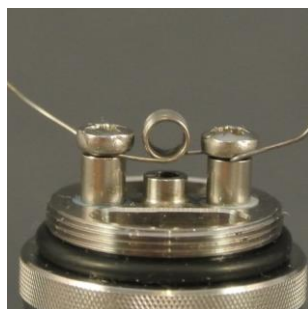
Pic. 6: The coil should now be exactly centered and floating about 1-1.5mm over the air hole.
