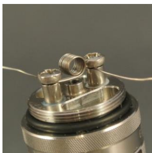
Pic. 5: The winding aid can now be removed.
