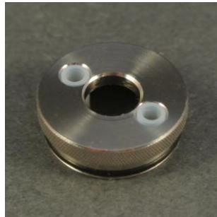
Pic. 6: On the top, both tubes should now be flush with the chamber cap.
