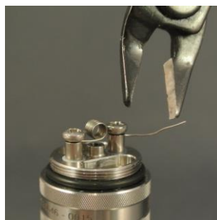
Pic. 7: Cut off excess wire on both sides.
