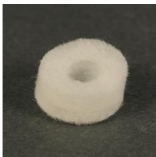
Pic. 1: The cylindrical wick pads are made from organic cotton and have a hole in the middle.
