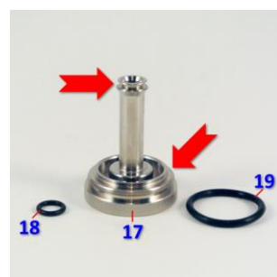
Pic. 20: The top cap and the chimney form a single unit [17]. In the recesses the o-rings [18,19] are attached.
