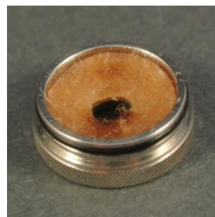
Pic. 8: Even after changing the actual coil, the cotton pad wick can still be used.
