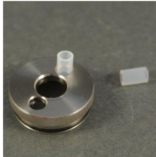
Pic. 2: These are pushed from above through the wick holes until they are stuck.
