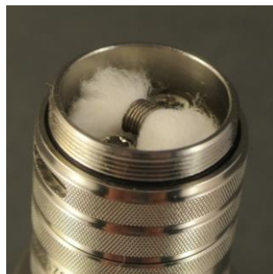
Pic. 14: The chamber sleeve is screwed carefully. The coil should not be displaced.
