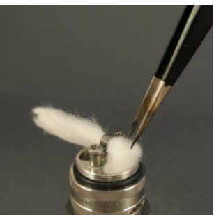
Pic. 12: The cotton should thereby fill the depression well, but by no means be stuffed into it.
