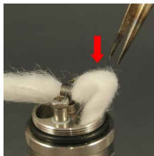
Pic. 11: Using tweezers, lead the cotton into the side recesses of the base.
