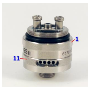
Pic. 9: The AFC-ring [11] should be fitted with easily rotating movements. Be careful not to damage the o-ring.
