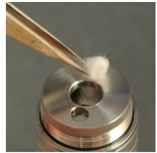
Pic. 4: These pieces are pushed through the wick holes.
