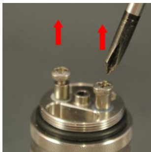
Pic. 1: First, the screws are loosened somewhat for the attachment of the coil.
