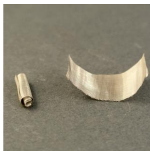
Pic. 2: The mesh is formed into a roll, which is then used as a wick. You should not roll the wick too tight.
