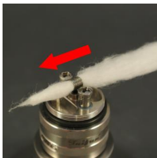
Pic. 9: Now you need a cotton strip about 5 cm long which is passed through the coil.
