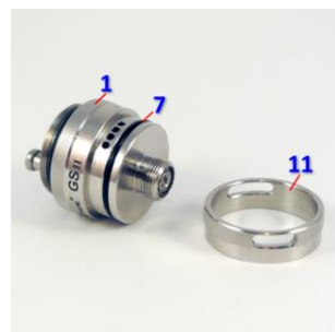
Pic. 8: The AFC ring [11] is placed on the base [1] and held there by the o-ring [7].
