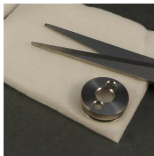
Pic. 11: For this you press the chamber cap on the cotton pad, and cut along the pressure point.
