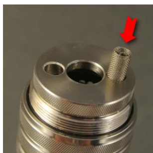
Pic. 5: The first roll is pushed in the chamber cap with slightly rotating movements. Do not apply pressure.
