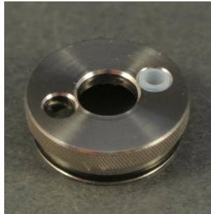
Pic. 3: The tubes are completely submerged in the chamber cap.
