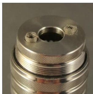
Pic. 7: Now cut the rolls approximately 1-2 mm above the chamber cap. Make sure not to deform the rolls.
