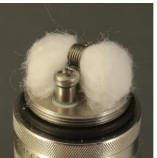
Pic. 13: A completed coil assembly should look like this.
