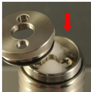
Pic. 15: Put the chamber cap at the chamber sleeve. The wick holes should land above the cotton.
