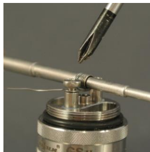
Pic. 3: The wire is placed under the screws. These are then tightened carefully.
