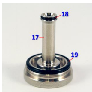
Pic. 21: The smaller o-ring [18] is used to seal against the chamber cap. The big o-ring [19] seals the tank.
